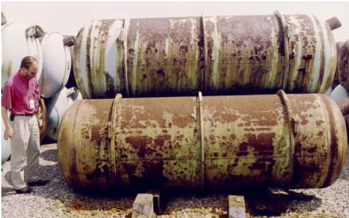
Depleted uranium storage cylinders at the Portsmouth (Ohio) Gaseous Diffusion Plant site. (U.S. DOE)
