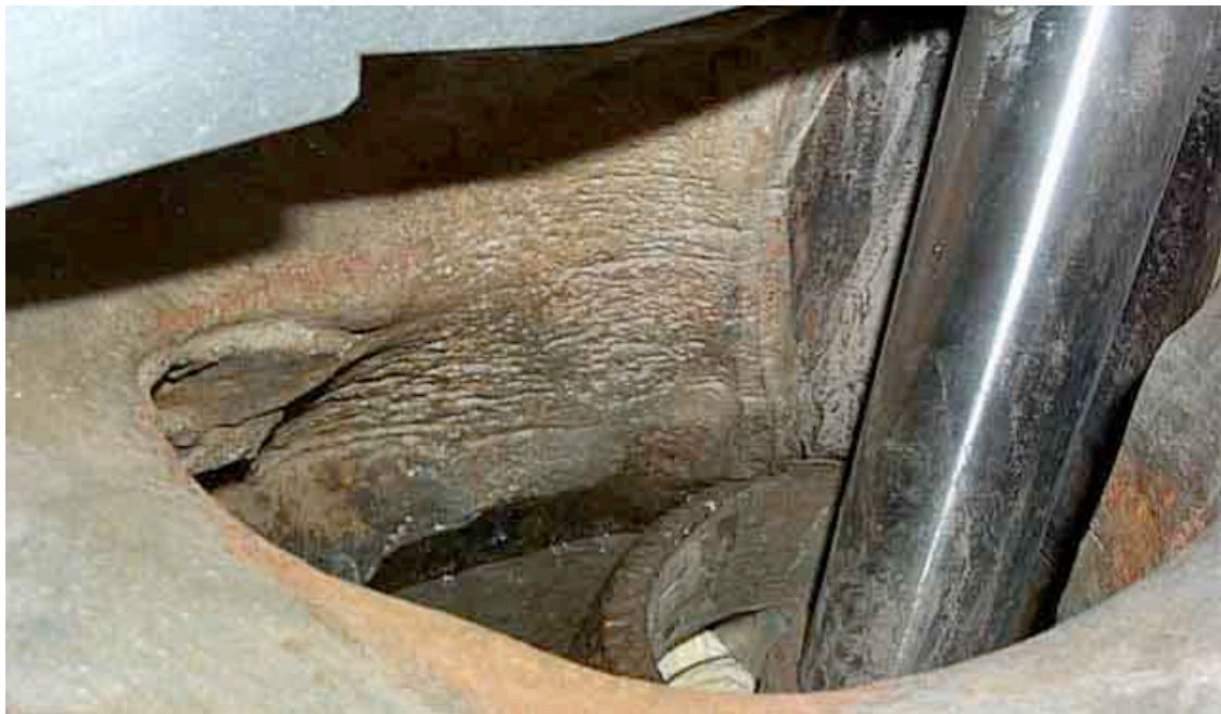
The large hole in the reactor vessel head around the vessel head nozzle.
