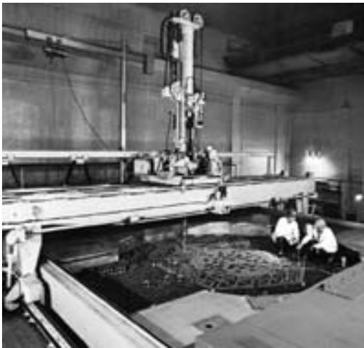
Figure 2.4. The BFS-2 Critical Assembly at the Institute of Physics and Power Engineering (IPPE), Obninsk, Russia, has huge inventories of HEU and plutonium. These include about 700 kg of weapon-grade uranium fuel in thousands of disks that are stacked up in columns mixed with similar disks of 36-percent enriched HEU, depleted uranium and plutonium to simulate large fast-reactor cores. Since the maximum enrichment in a fast reactor core is less than 36-percent, the weapon-grade uranium is not required and could be declared excess and blended down by the MCC Program. 80
