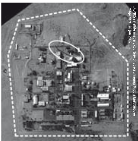
Figure 9.7. The Dimona nuclear complex in Israel. The on-site reprocessing plant has an estimated capacity of about 40–100 tons of spent fuel per year. The stack (revealed by its shadow) out of which krypton-85 would most likely be released, is marked by the white ellipse. The area enclosed by the dashed boundary, about 1000 meters at its widest point, indicates the fence of the secure area outside of which stand-off verification detectors could be placed. Based on the findings of the WAK case study, a few detectors located beyond the fence could make it virtually impossible for undeclared plutonium separation to evade detection over time.
