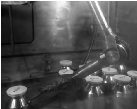
Figure 6.1. Bottles (left) being filled with plutonium-oxide in shielded glove-boxes (right) at Russia's Mayak RT-1 reprocessing plant. Most of Russia's 50
