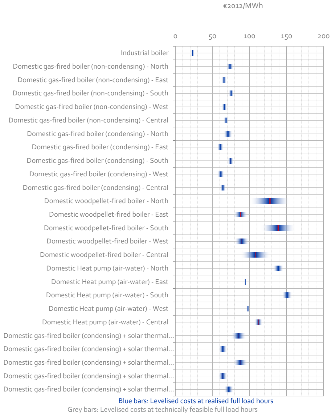
Figure 3-16: Levelised cost of heat in the EU28 for various technologies in the EU28
